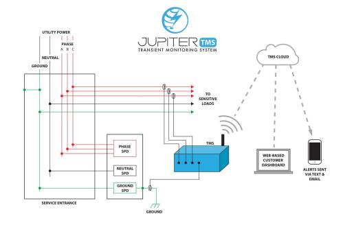
**Precision Timestamping:** Jupiter TMS timestamps detected transient with microsecond accuracy. When insurance claims are filed for damaged assets, Jupiter TMS provides the ground-truth proof that lightning was the source.
