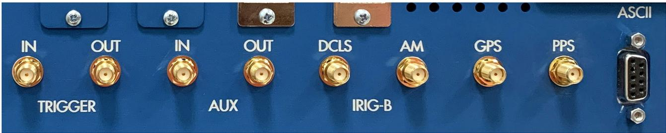
Figure 12: Jupiter TMS timing input connections on rear panel.
