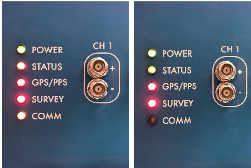
Figure 17: Jupiter TMS power front panel LED indicators during the boot process. At left, “Status” and “Comm” LEDs are briefly illuminated in orange near the end of the boot process. When the system is fully booted, armed, and ready to acquire data, the “Status” LED is illuminated in green (right).
