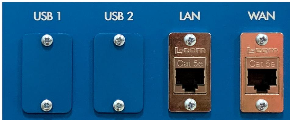
Figure 15: Jupiter TMS communications ports on the rear panel. This image shows the WAN port populated with the Ethernet option.
