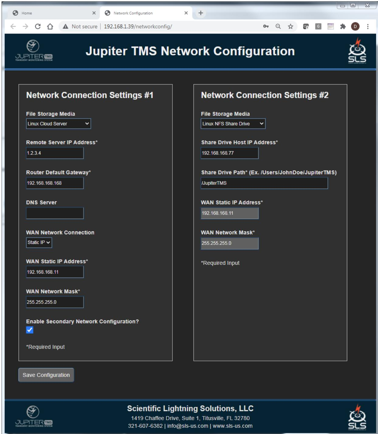
Figure 24: Jupiter TMS network configuration page with the secondary network connection interface enabled. In this case, the primary connection is set to a Linux Cloud Server and the secondary connection is set to a Linux NFS Share Drive. Note that the Static IP and Network Mask fields in the secondary connections are non-editable because they have been specified in the primary connection.
