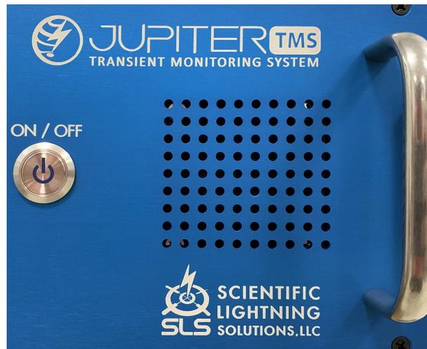
Figure 5: Jupiter TMS chassis cooling vents.
