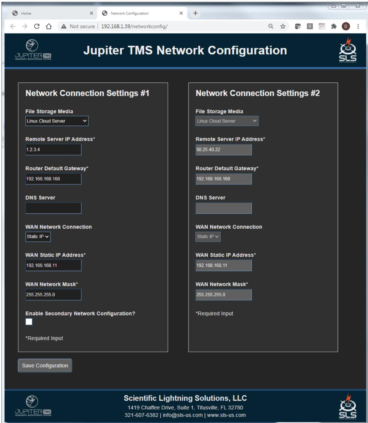
Figure 20: Jupiter TMS network configuration page, accessed via navigating to LANIP/networkconfig from a web-browser window on a computer connected to the Jupiter TMS LAN port. In this case, the Linux Cloud Server connection option and the Static IP network configuration are selected.
