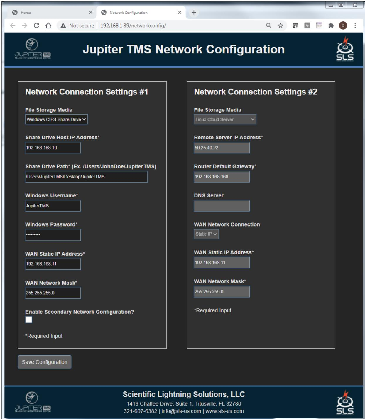
Figure 22: Jupiter TMS network configuration page, accessed via navigating to LANIP/networkconfig from a web-browser window on a computer connected to the Jupiter TMS LAN port. In this case, the Windows CIFS Share Drive option is selected.
