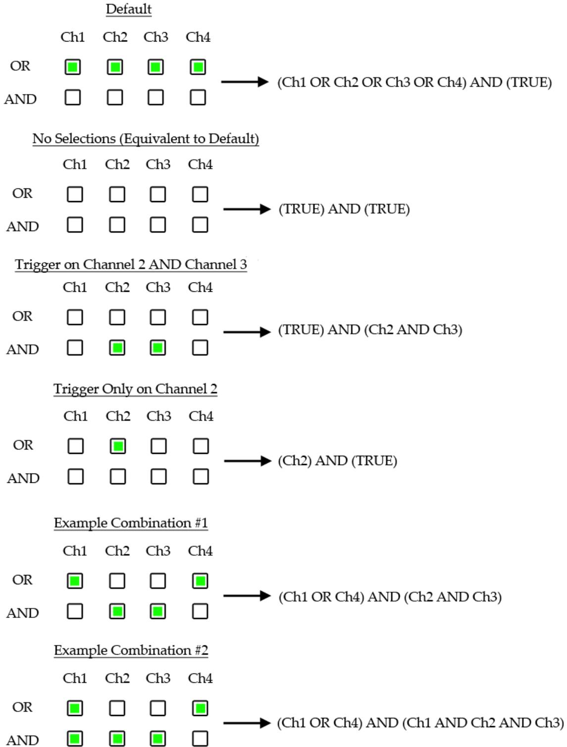
Figure 33: Illustration of Jupiter TMS logic trigger examples for basic and complex trigger schemes.
