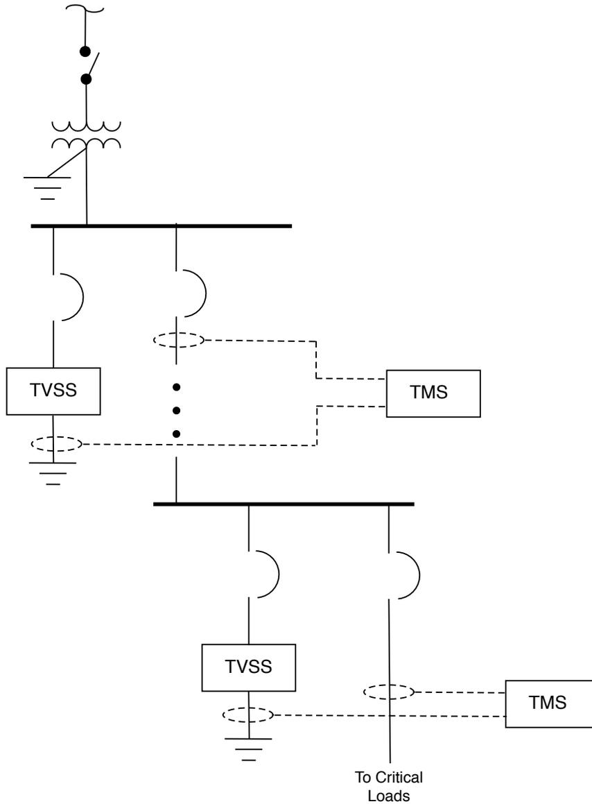
Figure 53: Single line diagram of Jupiter TMS installation including multiple units. This configuration can be used to accurately trace and pinpoint the origin of the injected surge.
