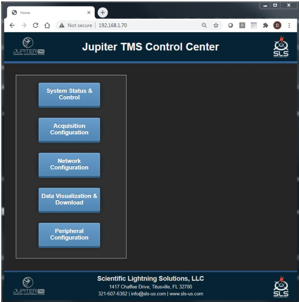
Figure 18: Jupiter TMS Control Center, accessed via navigating to the LAN port IP address from a web-browser window on a computer connected to the Jupiter TMS LAN port.
