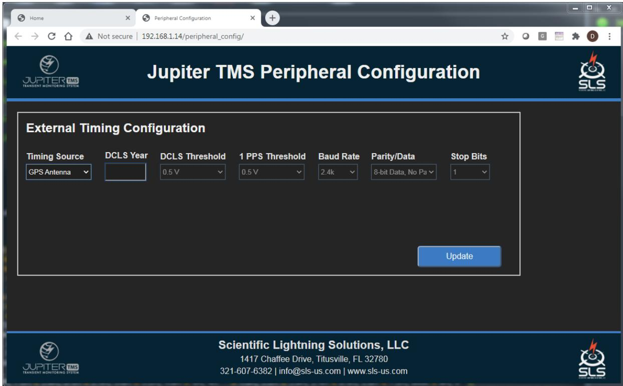
Figure 34: Screenshot of the Jupiter TMS Peripheral Configuration page with the GPS antenna timing source selected.
