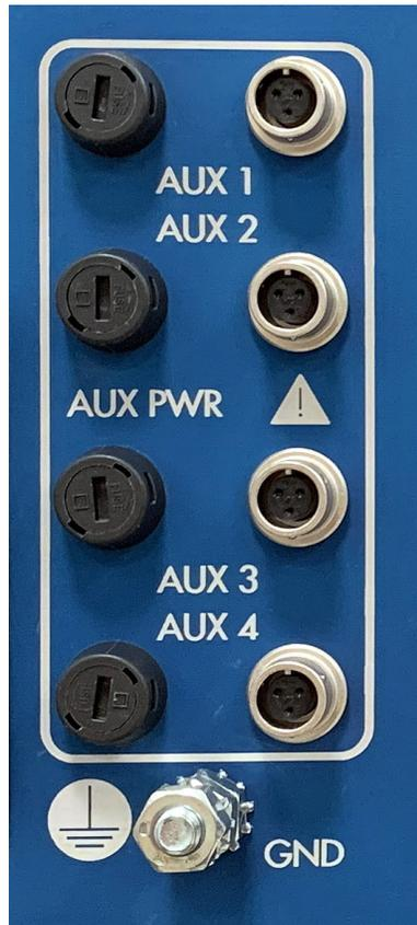
Figure 10: Jupiter TMS auxiliary power ports and chassis-mount fuse holders on rear panel.
