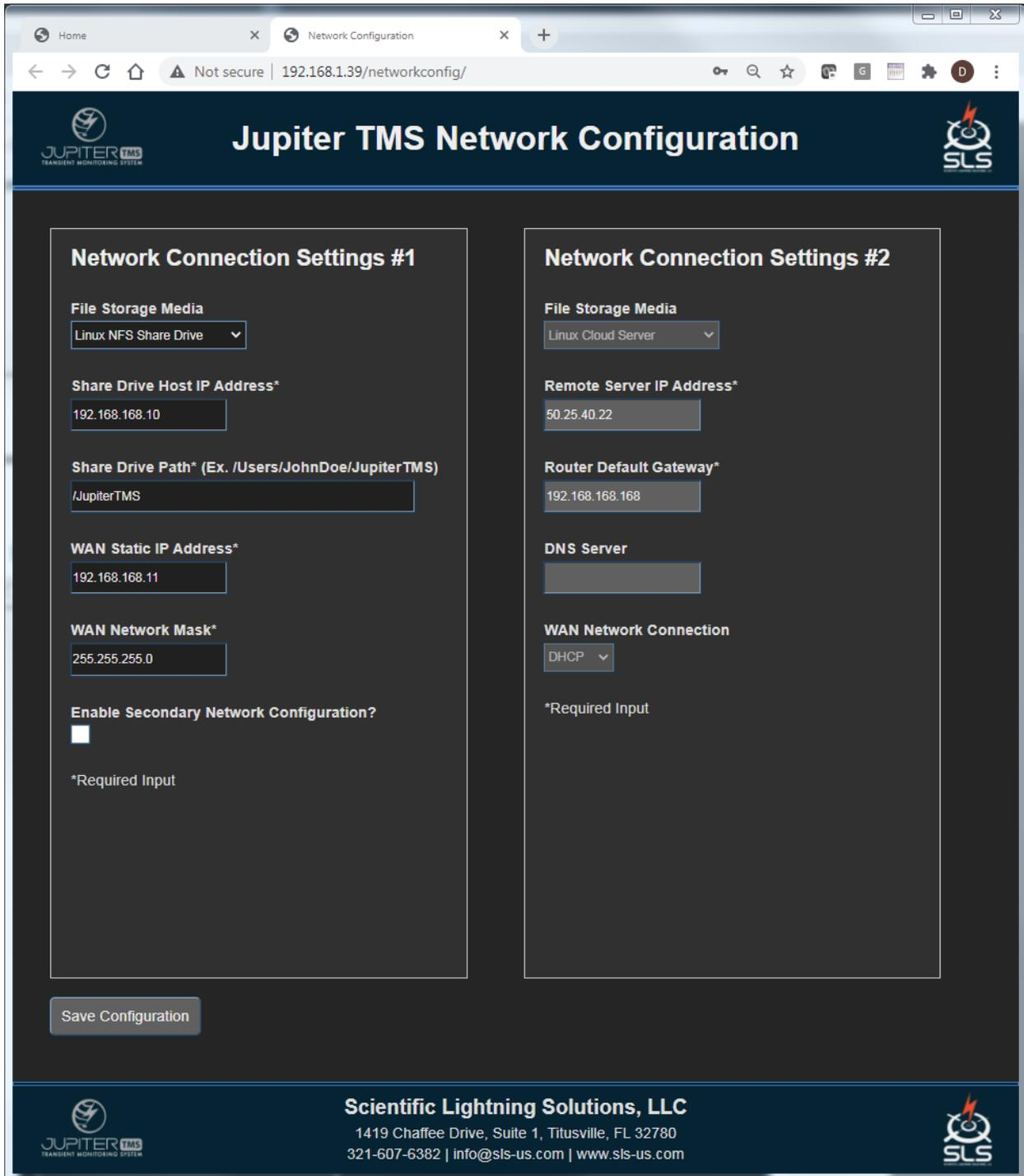
Figure 21: Jupiter TMS network configuration page, accessed via navigating to LANIP/networkconfig from a web-browser window on a computer connected to the Jupiter TMS LAN port. In this case, the Linux NFS Share Drive option is selected.
