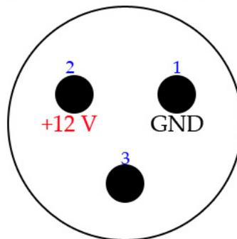
Figure 11: Jupiter TMS auxiliary power connector pin-out diagram.
