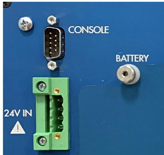
Figure 13: Jupiter TMS console connection on rear panel.
