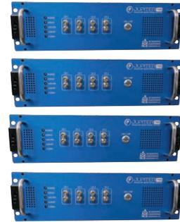
Each timing source can be used to provide accurate UTC timing for up to four Jupiter TMS Transient Monitoring Systems (or other peripheral instrumentation that accepts common timing inputs).
