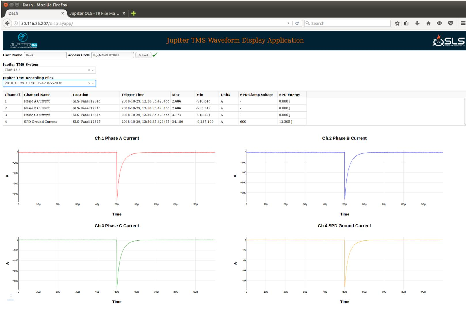
Figure 48: Jupiter TMS online waveform display application.
