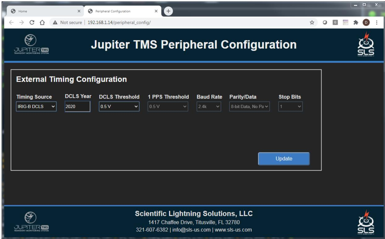
Figure 35: Screenshot of the Jupiter TMS Peripheral Configuration page with the IRIG-B DCLS timing mode selected and the year specified.
