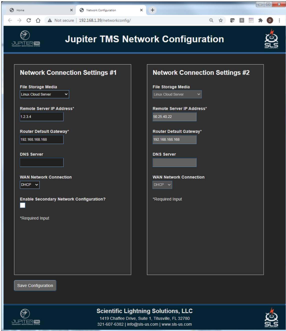
Figure 19: Jupiter TMS network configuration page. The page is accessed through the local Ethernet port on the rear panel of the Jupiter TMS chassis. In this case, the Linux Cloud Server connection option and the DHCP network connection are selected.
