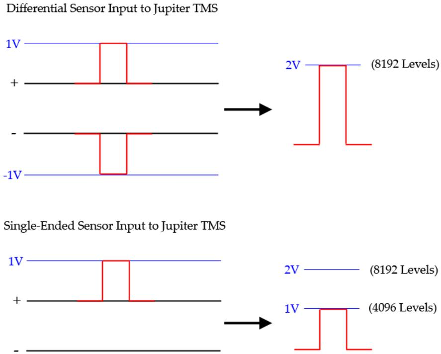
Figure 31: Illustration of Jupiter TMS differential versus single-ended input signals. For the single-ended input, the specified Trigger Level A must be below 1 V in order for the system to trigger.
