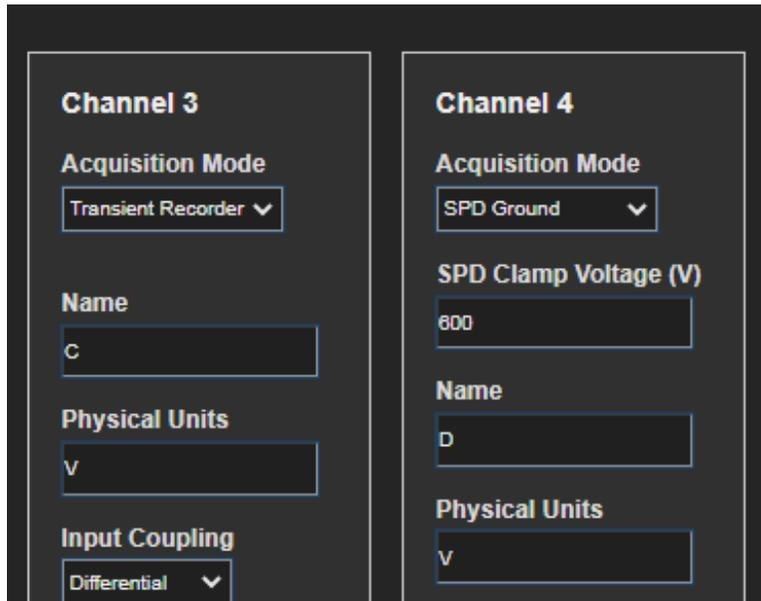
Figure 29: Jupiter TMS channel configuration interface page with SPD Ground Mode selected on Channel 4. Note the additional “SPD Clamp Voltage” numerical input field that was exposed when the SPD Ground Mode selection was activated.
