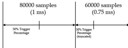
Figure 28: Illustration of LSP Jupiter TMS zero dead-time recording for consecutive triggers.
