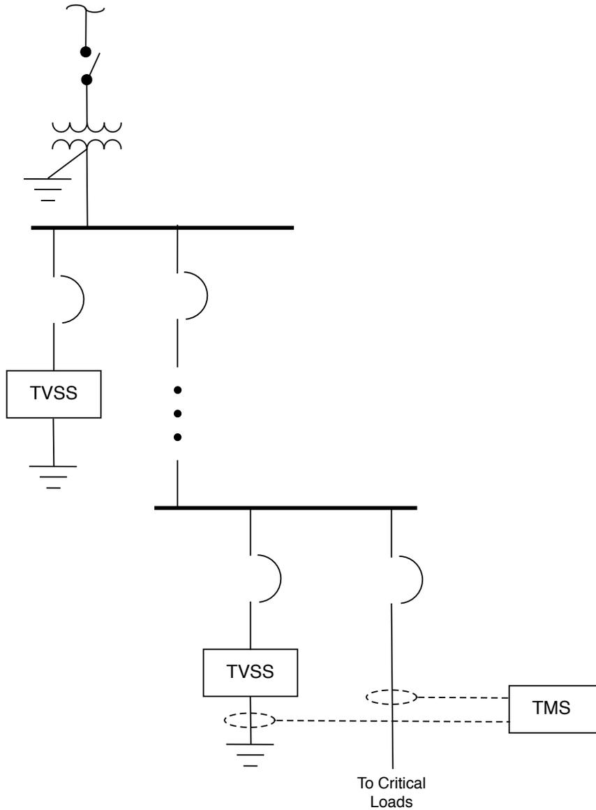
Figure 52: Single line diagram of Jupiter TMS installation on the last electrical panel before the critical loads. Jupiter TMS is used to monitor the three phase conductors and the SPD ground current.
