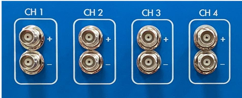
Figure 14: Jupiter TMS coaxial data acquisition input channels on the front panel.
