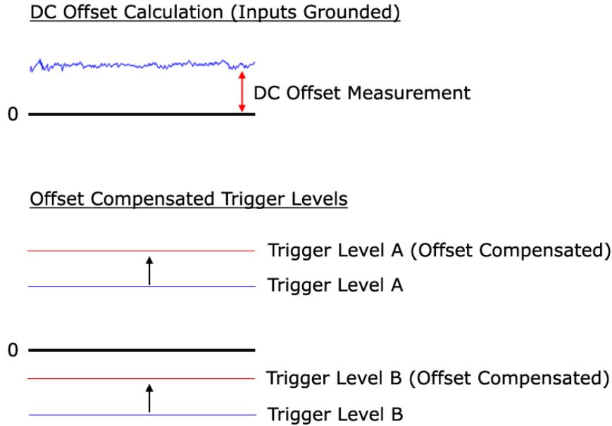
Figure 32: Illustration of Jupiter TMS automatic DC offset compensation for user-defined Trigger Level A and Trigger Level B.
