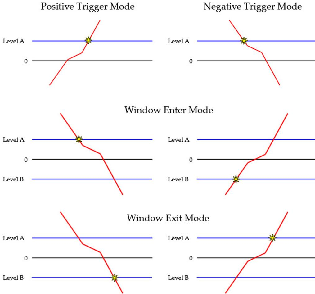
Figure 30: Illustration of Jupiter TMS trigger modes (positive, negative, window (enter), window (exit)). The yellow start indicates the time where the trigger would occur.
