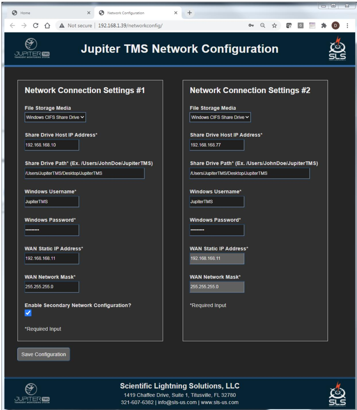
Figure 23: Jupiter TMS network configuration page with the secondary network connection interface enabled. In this case, both connections are configured to mount Windows CIFS share drives.
