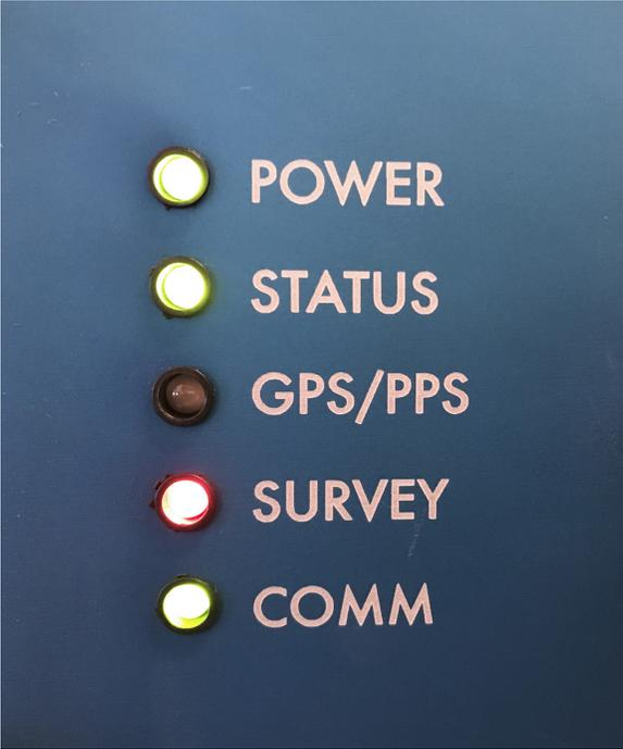
Figure 25: Jupiter TMS power front panel “Comm” LED is illuminated solid green when a successful connection has been established with the remote server or Linux/Windows share drive.
