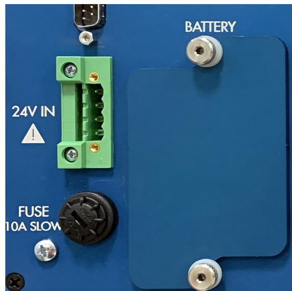
Figure 8: Jupiter TMS rear panel battery access cover.
