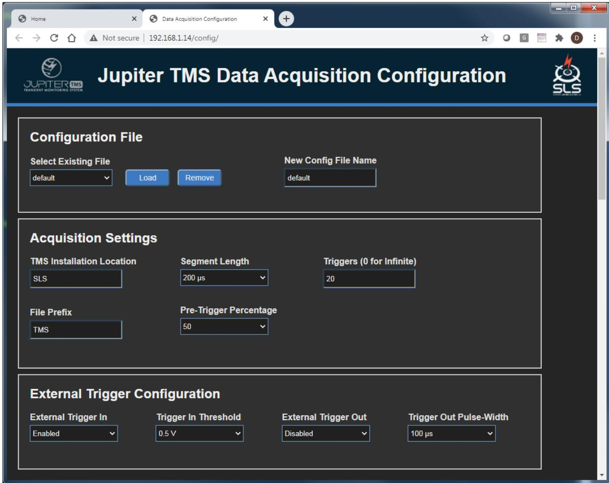
Figure 26: Jupiter TMS data acquisition configuration interface page.
