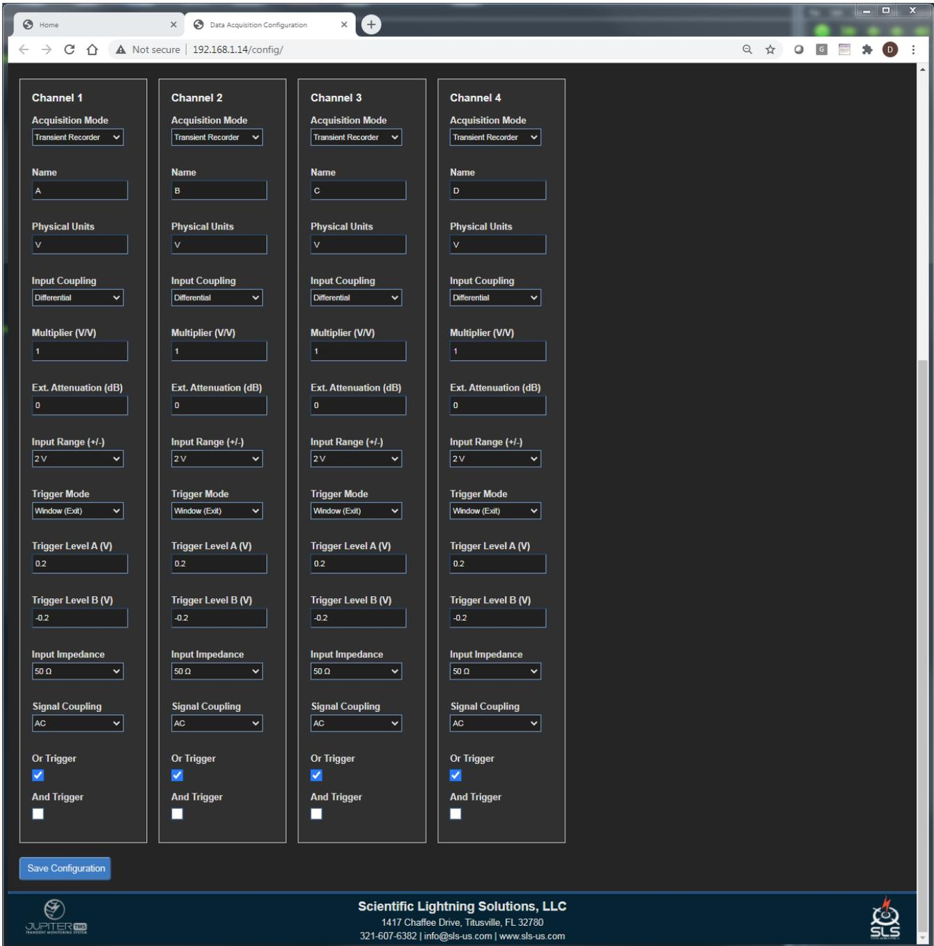
Figure 27: Jupiter TMS data acquisition configuration interface page.
