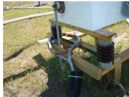
Figure 11. Two fiber loops (inside a garden hose) measuring current exiting the shunt resistor (box).
