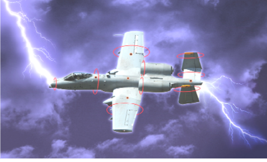
Figure 1. Fiber-optic Sensors Installations.
