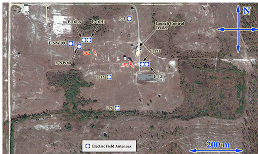
Figure 1. A Google Earth view of the ICLRT with the locations of the local electric field antenna network annotated. Electric field data used in this study were measured using electric field antennas E-7 and E-12 F. E-7, the southernmost antenna, is about 220 m from the field rocket launcher which is indicated by the red lightning bolt labeled LF2. E-12 F is about 180 m from the launcher.
